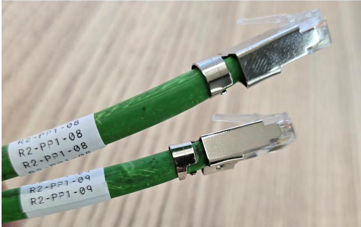
TAHAKOM HEAD OFFICE Riyadh (Cat.6A RJ-45 Connector)
